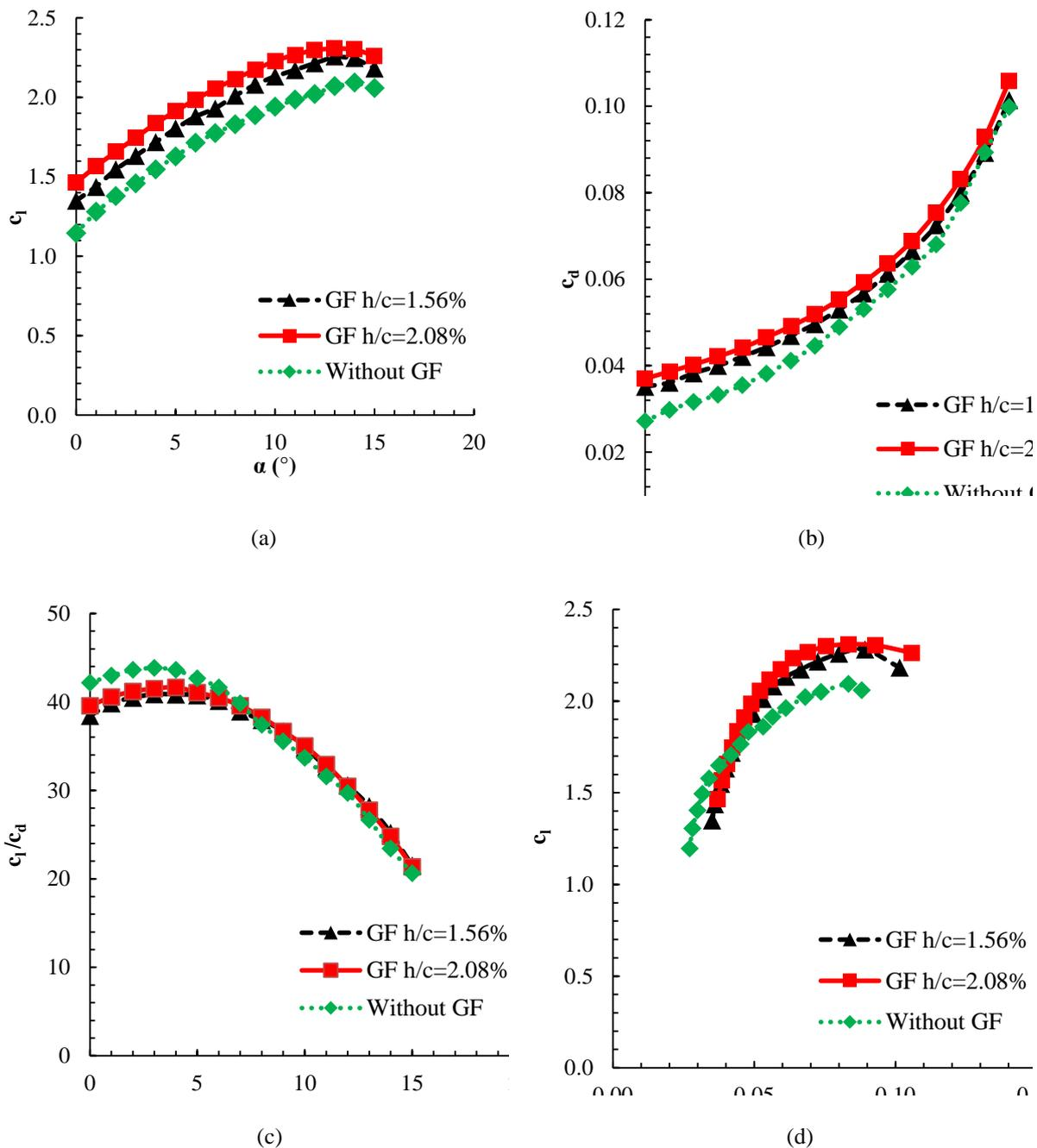
Figure 7. Comparison of aerodynamics coefficients of original aerofoil S1223 and aerofoil SELIG 1223 with gurney flap  $h/c=1.56\%$  and  $h/c=2.08\%$ : (a)  $C_l \times \alpha$ ; (b)  $C_d \times \alpha$ ; (c)  $C_l/C_d \times \alpha$  and (d)  $C_l \times C_d$
