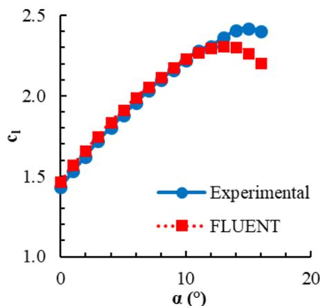
Figure 6. Comparison between experimental data and numerical results of the evaluation of lift coefficient  $c_l$  versus angle of attack  $\alpha$  for aerofoil S1223 with gurney flap  $h/c=2.08\%$  for  $Re=2.5 \times 10^5$
