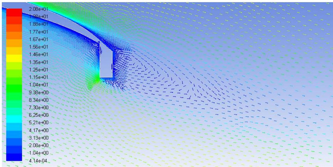
Figure 11. Detail of velocity field close to the trailing edge, with a gurney flap with  $h/c=2.08\%$ , showing the two counter-rotating vortices
