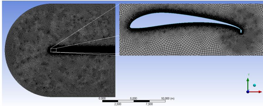
Figure 5. Mesh of SELIG 1223 aerofoil with a gurney flap  $h/c=2,08\%$  and an angle of attack  $\alpha=2^\circ$
