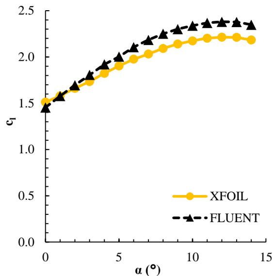
Figure 8. Lift polar diagrams of aerofoil S1223 with plain flap at  $x/c=80\%$  with a deflection angle of  $\delta=10^\circ$  computed with FLUENT and XFOIL codes for  $Re=2.5 \times 10^5$
