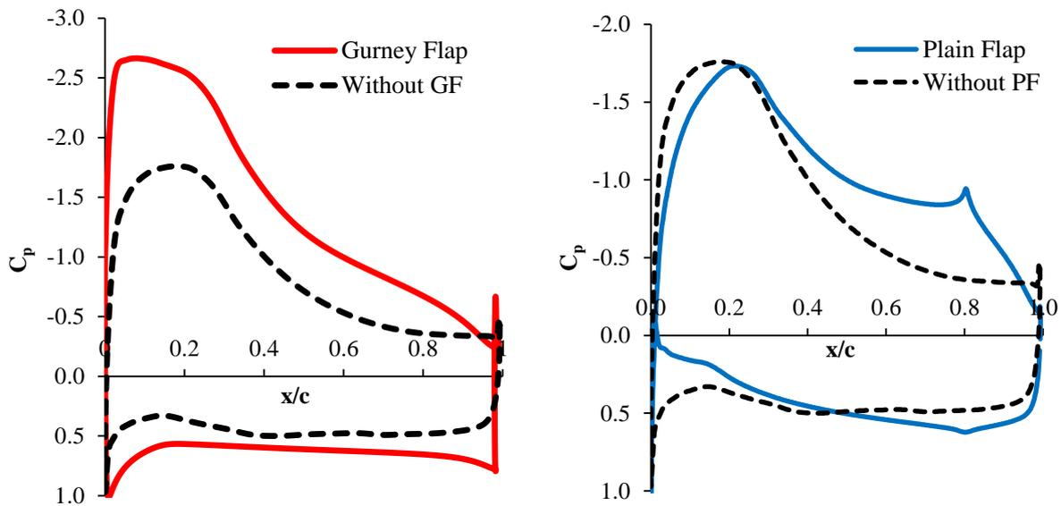
Figure 10. Comparison of pressure coefficient distributions over the aerofoil contour for  $Re=2.5 \times 10^5$ : (a) gurney flap  $h/c=2.08\%$  and (b) plain flap at relative distance of trailing edge  $x/c=20\%$  and  $\delta=5^\circ$
