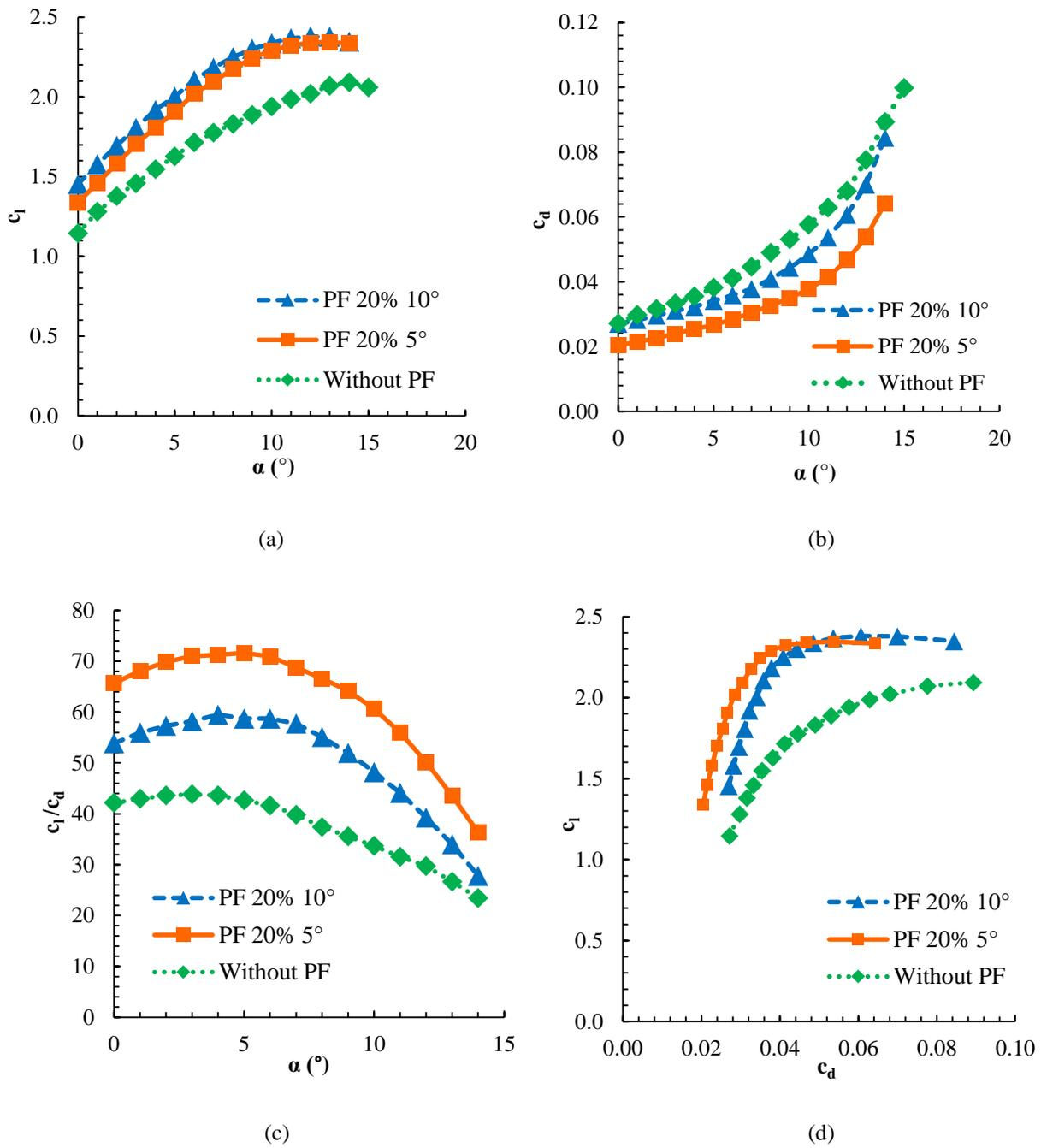
Figure 9. Comparison of aerodynamics coefficients of original aerofoil S1223 and aerofoil SELIG 1223 with plain flap at relative distance of trailing edge  $x/c=20\%$  and  $\delta=5^\circ$  and  $\delta=10^\circ$ : (a)  $c_l \times \alpha$ ; (b)  $c_d \times \alpha$ ; (c)  $c_l/c_d \times \alpha$  and (d)  $c_l \times c_d$
