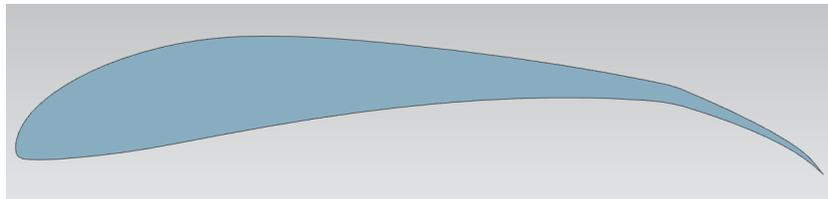
Figure 2. Aerofoil SELIG 1223 with plain flap at  $x/c = 80\%$  with a deflection angle of  $10^\circ$
